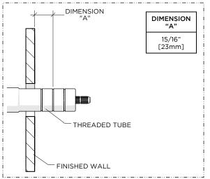
1. Remove the TILE GUARD when ready to install the TRIM then mark the THREADED TUBE in front of the finished wall at the length listed above.
