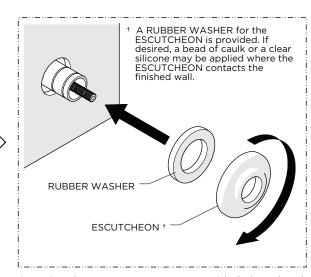
6. Using the RUBBER WASHER provided, thread and securely tighten the ESCUTCHEON onto the THREADED TUBE.
