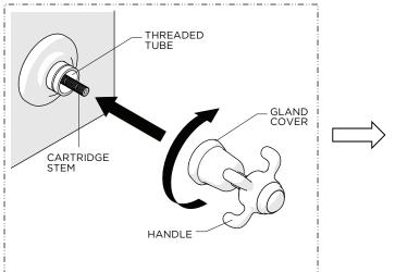
7. With the HANDLE in the desired orientation, thread and securely tighten the GLAND COVER onto the THREADED TUBE.
