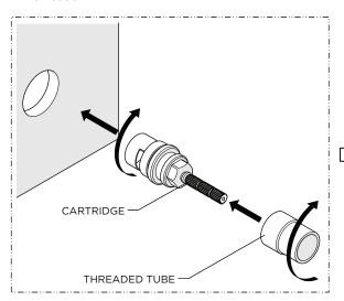
5. Thread and securely tighten the CARTRIDGE back into the VALVE and thread the THREADED TUBE back onto the CARTRIDGE then turn on the water supply and check for leaks.
