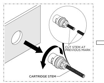
4. Remove the CARTRIDGE using a 21/32" [17mm] shower valve socket wrench (not provided) then cut the STEM at the previous mark.
